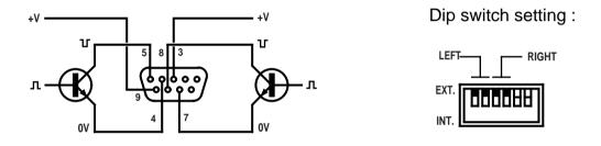
The dip switch setting is important to avoid a conflict between internal and external power supplies.
