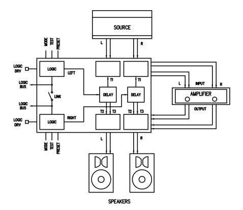
**3.1** Signal from the program source is muted by a dual reed relay. Output of the program source is left open while the input of the power amplifier is loaded with a low impedance RC network. From that point forward, there is no audio signal at the output of the power amplifier.
